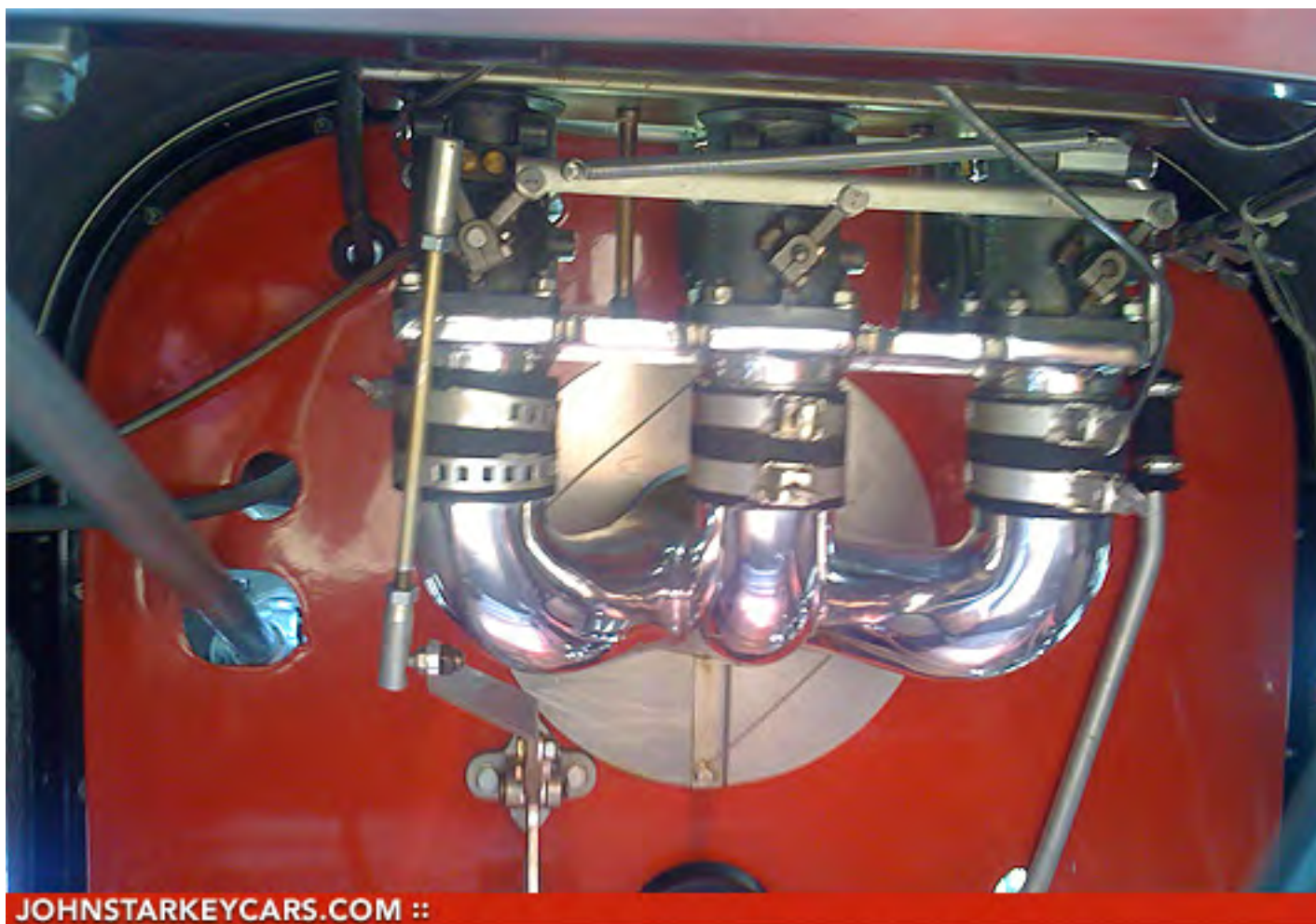
Inside the cockpit of the Miller Winfield Special are the three carburetors that feed the supercharger.
