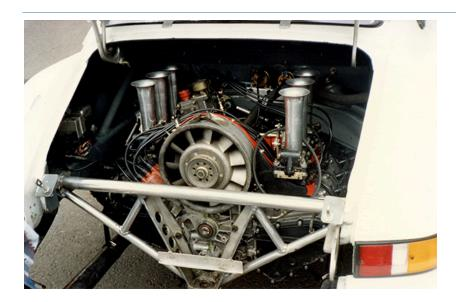
"I think the car is now roughly 50/50 tube frame to unitary chassis. All the bodywork, including the roof, is carbon fibre and the front end is a one-part K3 moulding. The front splitter is our design and has a wing cross sectional profile, the rear wing has a twisted chord and again is our own design, the car has a front diffuser with the air exiting from under the doors and the rest of the floor is completely flat, again made from carbon honeycomb sheet."
